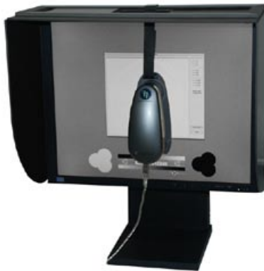
LCD-flat screen with ambient light hood and Eye-One Pro spectrophotometer.
