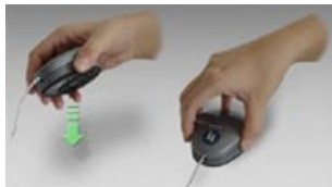
Calibration position for basICColor SQUID2 / Eye-One Display 2
