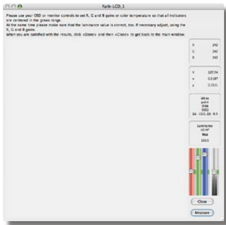
Measurement window for presetting the color temperature and the luminance of the monitor.
