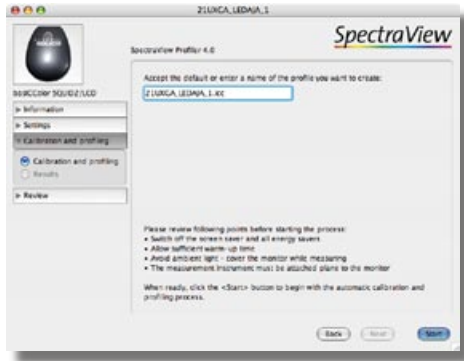
As the final setting before starting the calibration and profiling process a name for the ICC-profile has to be entered.
