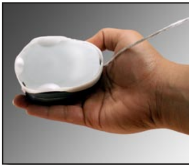
Positioning basicColor SQUID2 for ambient light measurement.
